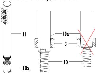
Important: The LEGS (I) have left-handed threads, therefore, it is necessary to rotate LEGS (I) counter-clockwise into BODY (5)
