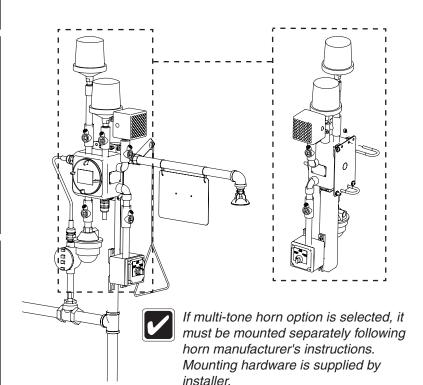
NOTICE! If the water supply line will be exposed to temperatures at or below freezing, the inlet supply must be freeze-protected 6 inches above the flow switch tee (freeze protection by others).
