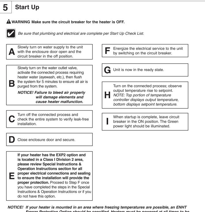
NOTICE! If your heater is mounted in an area where freezing temperatures are possible, an ENHT Freeze Protection Option should be specified. Heaters must be powered at all times to be Freeze Protected. If continuous power is not possible, do not allow the heater to remain full of water. Freezing of the heater can cause serious damage.
