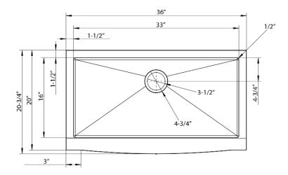
Dimensions of fixture are nominal and may vary within the range of tolerances established by ANSI Standard A112.19.2. Dimensions and specifications subject to change without notice.
